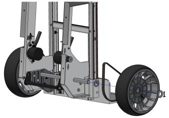
8. Use pliers to straighten and remove the cotter pins holding the wheels (B) on. Remove the wheel and belt (A) together.
