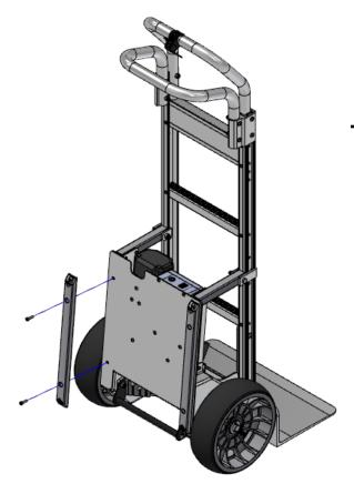
1. Remove pan head screws and the used wear strips.
